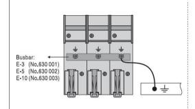
Multiple products installation, busbar E-3, E-5 or E-10 can be used to combine all the earth terminals to earth.
